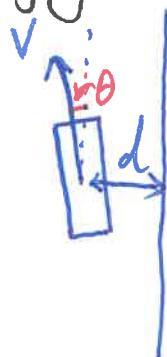
$$\begin{cases} d[n] = d[n-1] + \Delta T V \theta[n-1] & (\sin \theta \approx \theta) \\ \theta[n] = \theta[n-1] + \Delta T w[n-1] & (w[n] \text{ is the angular velocity}) \end{cases}$$
