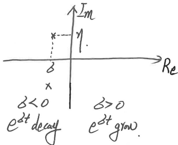
$$d(t) = C_1 e^{(\delta + j\eta)t} + C_2 e^{(\delta - j\eta)t}$$
