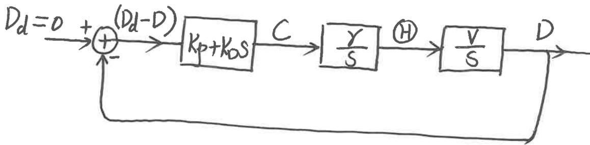
$$D = \frac{V}{s} \cdot \frac{\gamma}{s} \cdot (-K_p - K_D s) D \Rightarrow (s^2 + V \gamma K_D s + V \gamma K_p) D = 0$$
