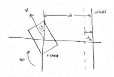
$$\frac{d}{dt} \begin{bmatrix} d(t) \\ \theta(t) \end{bmatrix} = \begin{bmatrix} V \sin \theta(t) \\ \omega(t) \end{bmatrix} \approx \begin{bmatrix} V \theta(t) \\ \omega(t) \end{bmatrix}$$
