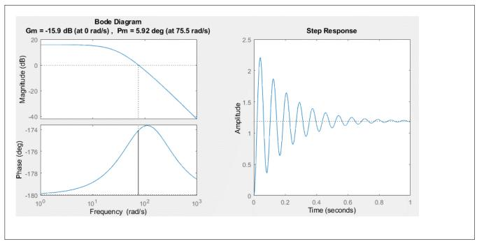
Part 2. The main issue with a PD controller is that it amplifies high frequency signals. If the physical system cannot dissipate high frequency disturbances effectively, then a PD controller may not perform well. Next, we will implement a lead controller. A lead controller can increase a system's phase margin without significantly amplifying high frequency signals. First, let's implement a lead controller in the form:
