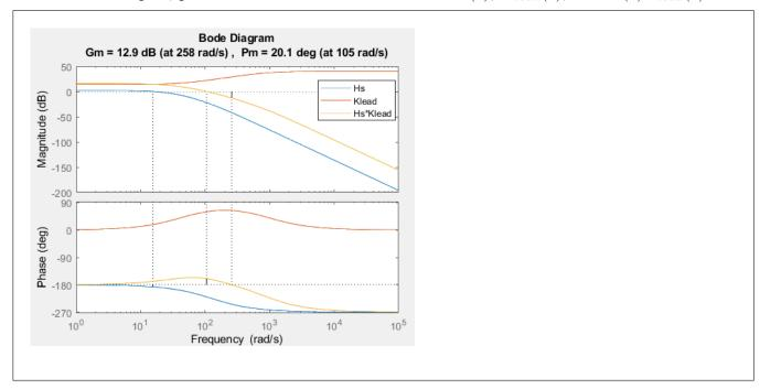
What is the phase margin of the open-loop system  $K_{lead}H(s)$ ? Is this a stable system?
