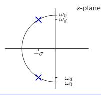
Find the frequency  $\omega$  at which the phase of the response y(t) is  $-\pi/2$  if  $x(t)=\cos\omega t$ .
