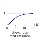
Let  $\omega_0$  represent the frequency where  $|H(j\omega_0)|=1$ . The system will be stable if the angle of  $H(j\omega_0)$  is greater than  $-\pi$  and unstable otherwise.  $K_p=33$
