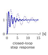
The loss of gain margin is severe when z = 0.4.
