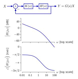
Consider the frequency response of an open-loop system  $H(s) = \frac{1}{s(s+1)(s+5)}$ .
