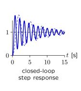
The loss of gain margin is severe when z=0.35.
