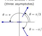
Mean Rule: If # of poles is at least two greater than the # of zeros, then the average closed-loop pole position is independent of  $K_p$ .
