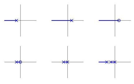
**Break-Away Rule:** Increasing  $K_p$  after two real-valued closed-loop poles collide causes them to split off the real axis.
