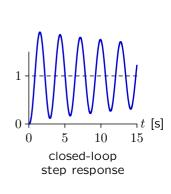
Let  $\omega_m$  represent the frequency where  $|K_pH(j\omega_m)|=1$ . When phase margin  $\to 0$ , the closed-loop response no longer converges.
