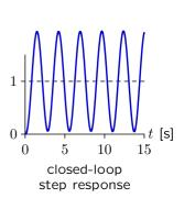
Let  $\omega_m$  represent the frequency where  $|K_pH(j\omega_m)|=1$ . When phase margin goes negative, the closed-loop system is unstable.
