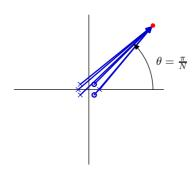
**High-Gain Rule:** If the # of poles exceeds the # of zeros by N, there will be N high-gain asymptotes with angles at  $(2n+1)\pi/N$ .
