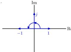
Multiplying by j rotates a vector by  $\pi/2$ . Multiplying by  $j^2 = -1$  rotates a vector by  $\pi$ .
