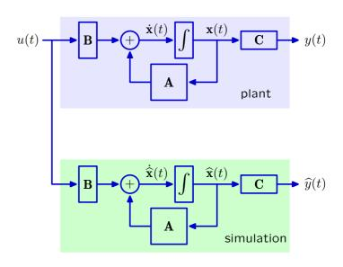
We embed both the plant and observer in state-space controllers, so that the simulation can provide estimates of the state  $(\hat{\mathbf{x}}(t))$  and input  $(\hat{u}(t))$ .
