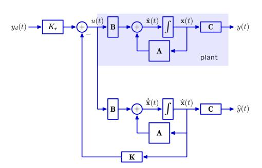
Unfortunately the resulting system is **feedforward**. It's utility depends critically on the accuracy of the match between the plant and observer.
