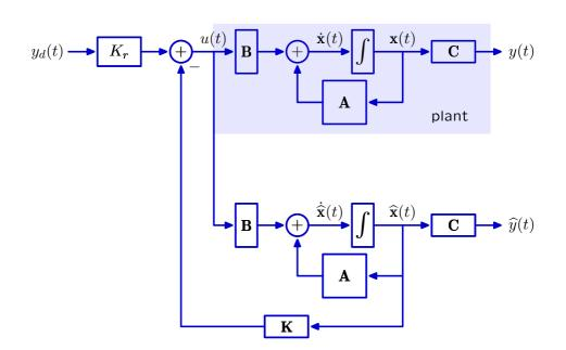
Fortunately, we can use **feedback** to measure and correct simulation errors! Calculate the difference between y(t) and  $\widehat{y}(t)$ .
