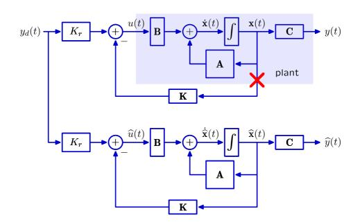
... we can substitute the simulated states  $\hat{\mathbf{x}}(t)$  for the missing states  $\mathbf{x}(t)$ . Similarly, we can substitute  $\hat{u}(t)$  for u(t) as well.
