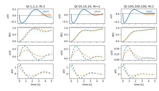
Increasing L's by increasing  $Q_l$ 's improves match (especially for  $\theta(t)$ ).
