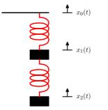
$$f_{m1} = m\ddot{x}_1(t) = k\left(x_0(t) - x_1(t)\right) - k\left(x_1(t) - x_2(t)\right) - b\dot{x}_1(t)$$
