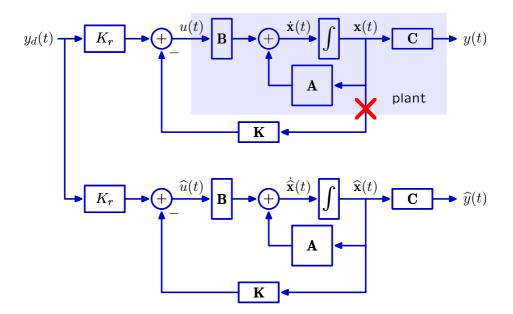
... we can substitute the simulated states  $\widehat{\mathbf{x}}(t)$  for the missing states  $\mathbf{x}(t)$ . Similarly, we can substitute  $\widehat{u}(t)$  for u(t) as well.
