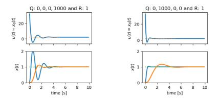
Left panels show results when feedback is from lower (output) mass only. Right panels show results when feedback is from upper (internal) mass only.
