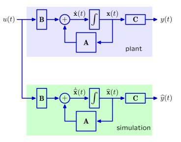
We can build state-space **controllers** for both the plant and the simulation. The simulation then provides estimates of the state  $(\hat{\mathbf{x}}(t))$  and input  $(\hat{u}(t))$ .
