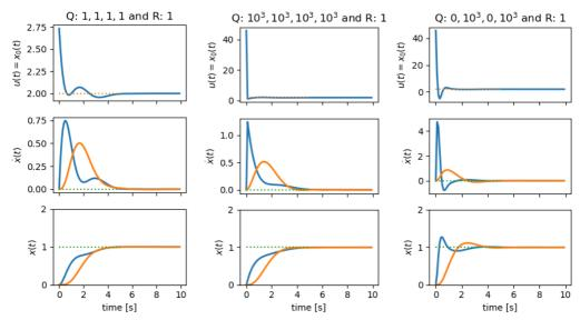
Increasing all values of  ${\bf Q}$  doesn't have a big effect. Setting  ${\bf Q}$  to zero for velocity terms increases speed and overshoot.
