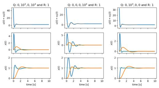
Reducing  $x_1$  cost causes large change in  $x_1$  and faster convergence of  $x_2$ . Reducing  $x_2$  cost speeds  $x_1$  with little effect on  $x_2$ .
