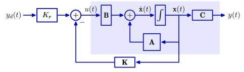
The closed-loop poles of a state-space model are equal to the roots of its characteristic polynomial:
