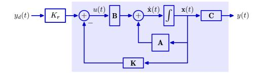
This method uses  $K_r$  to anticipate and pre-correct unwanted offsets in the rest of the system.
