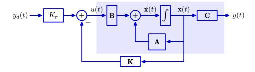
Matrices A, B, and C constitute a **model of the plant** (shaded).
