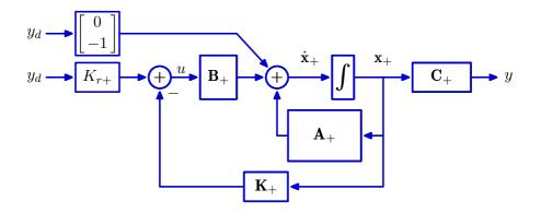
Express both the original system equations and the tracking equation as a first-order matrix equation in the augmented state.
