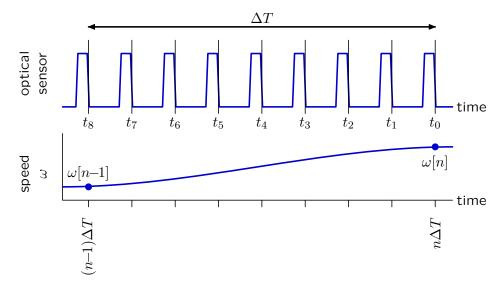
Let  $\widetilde{\omega}$  represent our estimate of angular speed based on the experimentally determined times  $t_i$ . If ticksperestimate=8, the time for 8 pulses to occur is equal to the time for one turn of the rotor (since there are 8 blades on the rotor). Therefore the angular speed is approximately 1 revolution divided by the time for 8 pulses of light:
