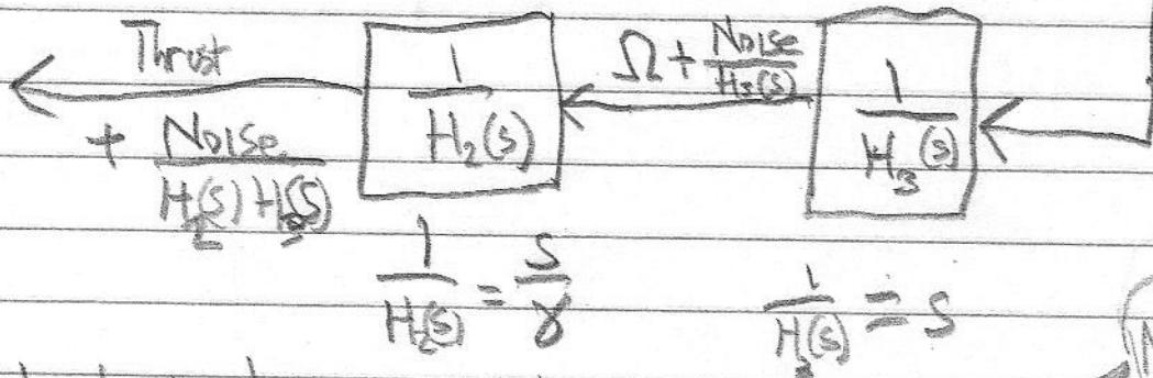
$$|w| = \left| \frac{1}{H_2(jw)} \right| = \left| \frac{1}{H_1(jw) H_3(jw)} \right| = \left| \frac{w^2}{8} \right|$$
