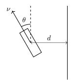
$$\begin{split} d[n] &= d[n-1] + \Delta T \nu \theta[n-1], \\ \theta[n] &= \theta[n-1] + \Delta T \underbrace{\omega[n-1]}_{\text{we control}}. \end{split}$$
