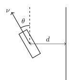
$$\begin{bmatrix} d[n] \\ \theta[n] \end{bmatrix} = \underbrace{\begin{bmatrix} 1 & \nu \Delta T \\ -K_p \Delta T & 1 \end{bmatrix}}_{A} \begin{bmatrix} d[n-1] \\ \theta[n-1] \end{bmatrix}$$
