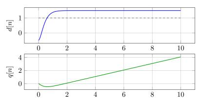
q[n] accumulates the distance error over time.
