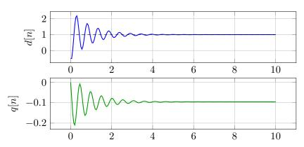
q[n] accumulates the distance error over time.
