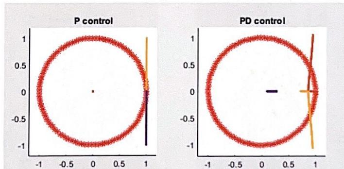
Here the red circle indicates the unit circle in the complex plane. We observe P control is unstable because the natural frequencies are outside of the unit circle regardless of the K<sub>p</sub> values we pick. For the case of PD control, there are cases where all 3 natural frequencies are within the unit circle, which implies the system is stable.
