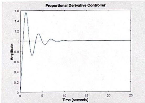
Based on this simulation result, we observe that the PD controller is stable. The car can follow a line with no steady-state error. Next, we can use the MATLAB tools to study stability and optimize the values of Kp and Kd.
