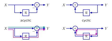
**Feedforward** systems contain no cyclic pathways. Their responses consist of a sum of components: each characterized by an aggregate gain and delay.
