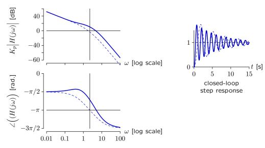
The loss of gain margin is severe when z = 0.35.
