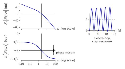
Gain and phase margins provide useful stability metrics that can be computed directly from the open-loop frequency response.  $K_p = 1$
