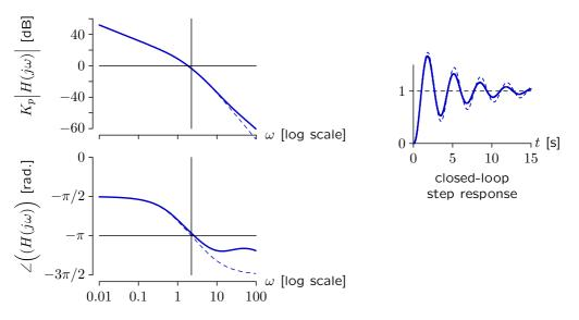
Moving the compensator to a lower frequency increases convergence rate.  ${\cal K}_p=20$
