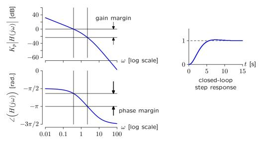
Gain and phase margins provide useful stability metrics that can be computed directly from the open-loop frequency response.
