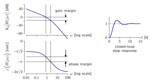
Gain and phase margins provide useful stability metrics that can be computed directly from the open-loop frequency response.  $K_p = 10$
