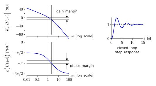
Gain and phase margins provide useful stability metrics that can be computed directly from the open-loop frequency response.  $K_p = 20$
