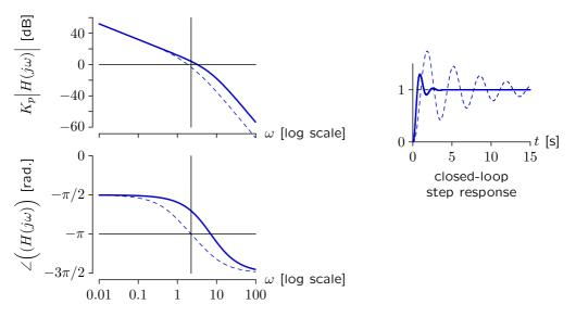
The loss of gain margin is severe when z = 0.5.
