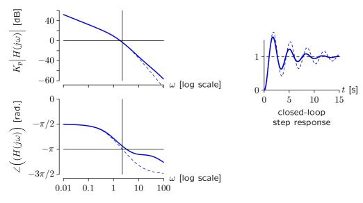
Moving the compensator to a lower frequency increases convergence rate.  $K_p = 20\,$
