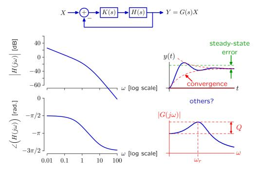
Design a controller based **solely** on the frequency response of the plant.
