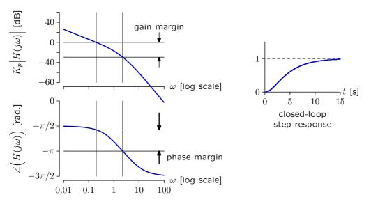
Gain and phase margins provide useful stability metrics that can be computed directly from the open-loop frequency response.  $V_{\rm c} = 2$
