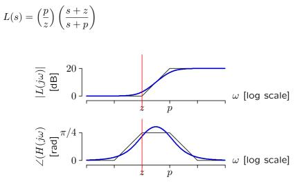
When adjusted appropriately, the increase in phase margin can more than compensate for the slight loss of gain margin.
