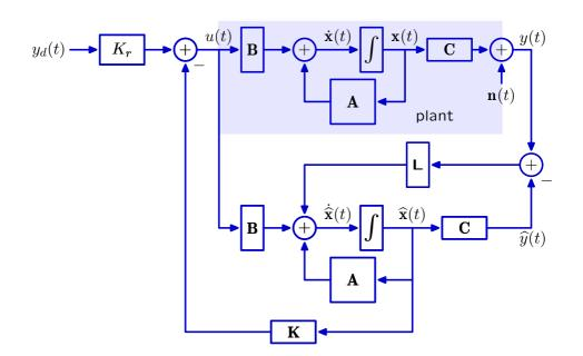
Compare a simple state-space controller with an observer-based controller.
