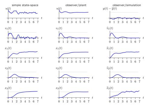
Compare a simple state-space controller with an observer-based controller.
