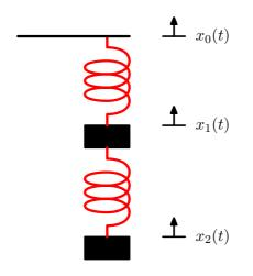
The goal was to move the input  $u(t)=x_0(t)$  so as to position the bottom mass  $y(t)=x_2(t)$  at some desired location  $y_d(t)$ .
