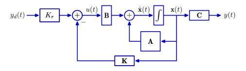
We can find  ${\bf K}$  using pole placement:
