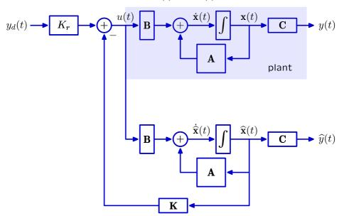
Fortunately, we can use **feedback** to correct simulation errors! Calculate the difference between y(t) and  $\hat{y}(t)$ .
