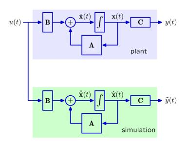
We can build state-space controllers for both the plant and the simulation.
