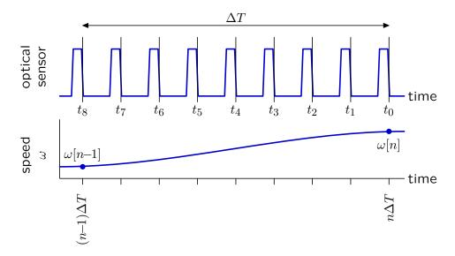
Let  $\tilde{\omega}$  represent our estimate of angular speed based on the experimentally determined times  $t_i$ . If **ticksperestimate=8**, the time for 8 pulses to occur is equal to the time for one turn of the rotor (since there are 8 blades on the rotor). Therefore the angular speed is approximately 1 revolution divided by the time for 8 pulses of light:
