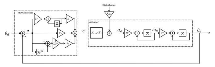
Determine the disturbance transfer function  $H_{dist}$  as follows
