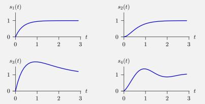
Which if any of the systems could have just one pole?  $\bf 1$  Which must have >1 but no more than 2 poles (both real)?  $\bf 2,3$
