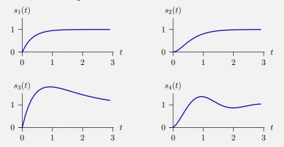
Which if any of the systems could have just one pole? Which must have >1 but no more than 2 poles (both real)?
