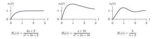
Only  $s_1(t)$  can be written as a single exponential, and only  $H_c(s)$  has a single pole. Therefore  $H_c(s)$  corresponds to  $s_1(t)$ .
