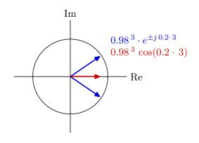
Output of a system with poles at  $z = re^{\pm j\Omega}$ .
