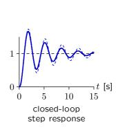
Moving the compensator to a lower frequency increases convergence rate.
