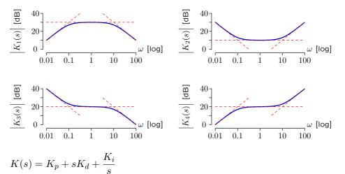
If  $K_d$  is nonzero, then the frequency response is large at high frequencies. If  $K_i$  is nonzero, then the frequency response is large at low frequencies.  $\to K_2(s)$
