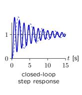
The loss of gain margin is severe when z = 0.35.
