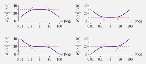
Which could correspond to a PID controller?
