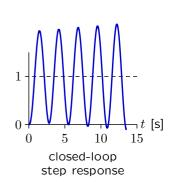
Let  $\omega_0$  represent the frequency where  $|H(j\omega_0)|=1$ . The system will be stable if the angle of  $H(j\omega_0)$  is greater than  $-\pi$  and unstable otherwise.  $K_v=1$
