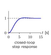
Let  $\omega_0$  represent the frequency where  $|H(j\omega_0)|=1$ . The system will be stable if the angle of  $H(j\omega_0)$  is greater than  $-\pi$  and unstable otherwise.  $K_v=5$
