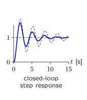
Moving the compensator to a lower frequency increases convergence rate.
