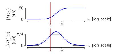
When adjusted appropriately, the increase in phase margin can more than compensate for the slight loss of gain margin.
