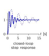
The loss of gain margin is severe when z = 0.4.
