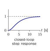
Let  $\omega_0$  represent the frequency where  $|H(j\omega_0)|=1$ . The system will be stable if the angle of  $H(j\omega_0)$  is greater than  $-\pi$  and unstable otherwise.  $K_v=2$
