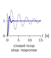
The loss of gain margin is severe when z = 0.5.
