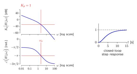
Let  $\omega_a$  represent the frequency where  $\angle(H(j\omega_a) \text{ is } -\pi.$  The gain margin is about 32 dB.
