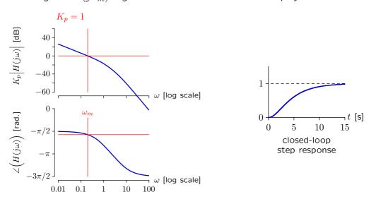
Let  $\omega_m$  represent the frequency where  $|K_pH(j\omega_m)| = 1$ . The phase margin is almost  $\pi/2$ .
