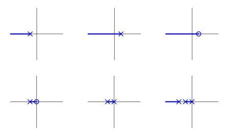
**Break-Away Rule:** Increasing  $K_p$  after two real-valued closed-loop poles collide causes them to split off the real axis.
