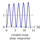
Let  $\omega_m$  represent the frequency where  $|K_pH(j\omega_m)| = 1$ . The angle of  $H(j\omega_m)$  is greater than  $-\pi$  so the closed-loop system is stable.
