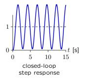
Let  $\omega_m$  represent the frequency where  $|K_pH(j\omega_m)| = 1$ . When phase margin goes negative, the closed-loop system is unstable.
