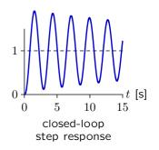
Let  $\omega_a$  represent the frequency where  $\angle(H(j\omega_a) \text{ is } -\pi)$ . When gain margin  $\rightarrow 0$ , the closed-loop response no longer converges.
