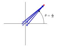
**High-Gain Rule:** If the # of poles exceeds the # of zeros by N, there will be N high-gain asymptotes with angles at  $(2n+1)\pi/N$ .
