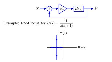
Given an expression for H(s), we can easily calculate the poles of the closed-loop system function G(s) numerically.
