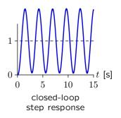
Let  $\omega_a$  represent the frequency where  $\angle(H(j\omega_a) \text{ is } -\pi)$ .
