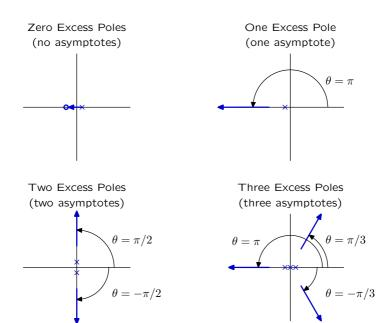
**Mean Rule:** If # of poles is at least two greater than the # of zeros, then the average closed-loop pole position is independent of  $K_p$ .
