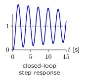
Let  $\omega_m$  represent the frequency where  $|K_pH(j\omega_m)| = 1$ . When phase margin  $\rightarrow 0$ , the closed-loop response no longer converges.
