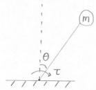
We want to stabilize this pendulum through applying a torque  $\tau$ . The system output is the measured angle  $\theta$ . First, using Newton's second law, we can write a differential equation that describes this system:
