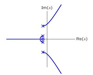
Track the open-loop poles as the gain  $K_p$  increases with  $K_d = K_p/0.7$ .
