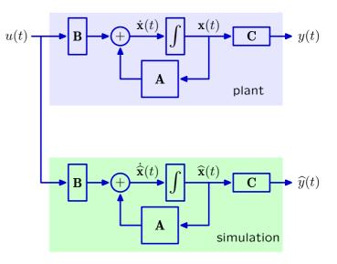
We can build state-space **controllers** for both the plant and the simulation. If our model of the plant (**A**, **B**, **C**) is perfect, then  $\hat{\mathbf{x}}(t) = \mathbf{x}(t)$  and  $\hat{y}(t) = y(t)$ .
