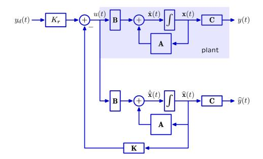
Fortunately, we can use **feedback** to correct simulation errors! Calculate the difference between y(t) and  $\hat{y}(t)$ . Then use that signal (times L) to correct  $\hat{\mathbf{x}}(t)$ .
