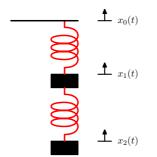
$$f_{m1} = m\ddot{x}_1(t) = k\Big(x_0(t) - x_1(t)\Big) - k\Big(x_1(t) - x_2(t)\Big) - b\dot{x}_1(t) - mg$$
