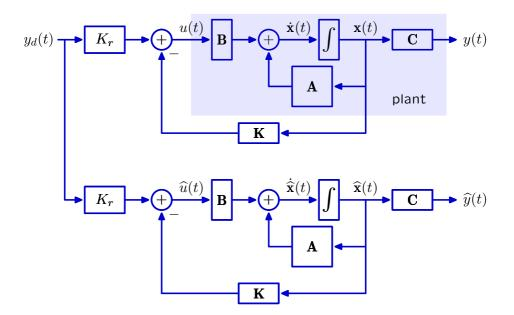
Recall the problem with designing a state-space controller for the twosprings system: the plant did not provide outputs for all of the states  $\mathbf{x}(t)$ .
