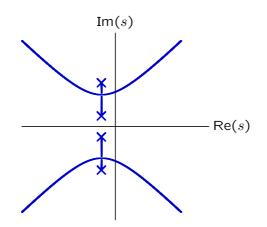
Track the open-loop poles as the gain K increases, starting at zero.
