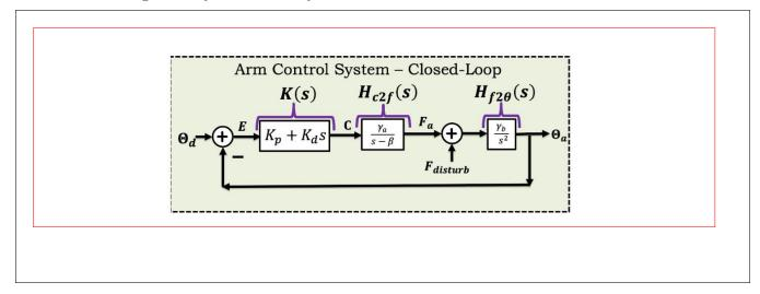
Based on this block diagram, please write the plant transfer function H(s).
