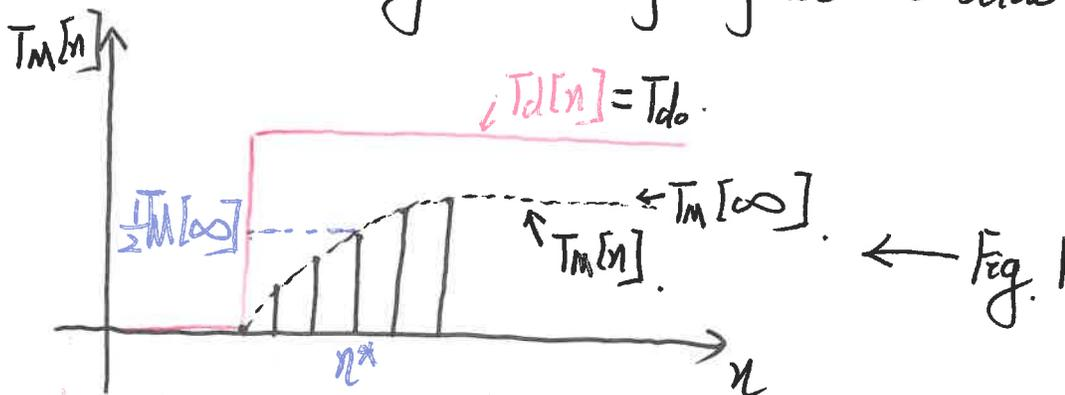
How to extract  $\beta$  (dissipation rate) and  $\gamma$  (actuator efficiency)?
