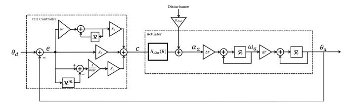
Determine the disturbance transfer function  $H_{dist}$  as follows
